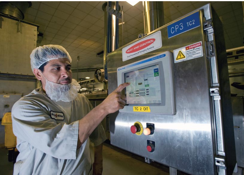
Arturo Lopez, tortilla chip operator, tracks the progress of one of the three tortilla chip lines on a PLC-controlled machine.
